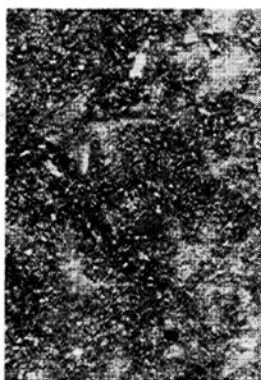
Fig. 12. Phosphate coating on oxide-covered surface without ultrasonic radiation. (5 min) ( \times 180 )
